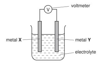
Which two metals produce the highest reading on the voltmeter?
